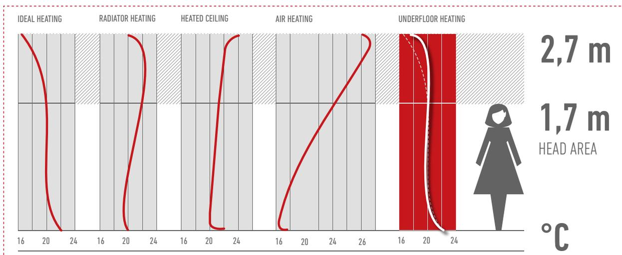
An underfloor heating is closest to an ideal heating regarding the vertical heat differences. Panel heatings are energy efficient and ideally suited for the use of renewable energies due to their very low flow temperature level. They create a maximum of comfort.
