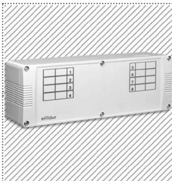
terminal block within box for wiring of up to 8 room thermostats and a maximum of 4 actuators per channel, type of protection IP 20, grey
