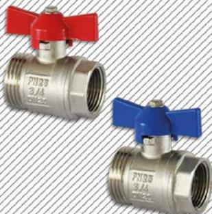
2x ball valve 3/4" female thread x 1" male thread, flat sealing, connection horizontal, among others for the shut off of flow and return of the pre-distributor HKV-VA, installation length = 50 mm
