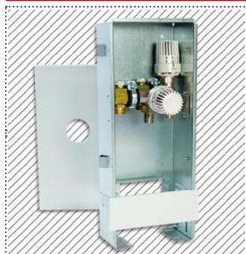
for single room control via thermostatic valve and limiting of the return temperature via RTL valve, built-in box with cover white, with opening for thermostat, incl. thermostatic valve pointing to the front and RTL valve with thermostat for areas of up to 16 m<sup>2</sup>\*
