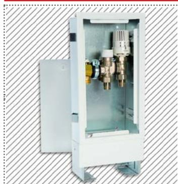
for single room control via thermostatic valve and limiting of the return temperature via RTL valve, built-in box with cover white, closed, incl. bottom part of thermostatic valve (prepared for actuator connection thread M30 x 1,5; not included) and RTL valve with thermostat, for areas of up to 16 m<sup>2</sup>\*
