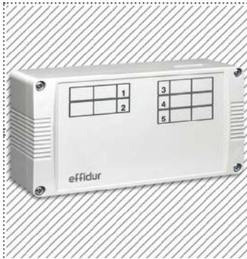
terminal block within box for wiring of up to 5 room thermostats and a maximum of 4 actuators per channel, type of protection IP 65, grey
