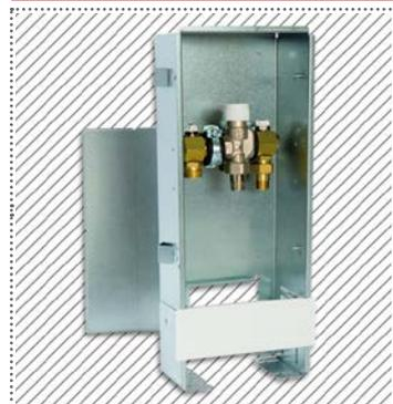
for single room control via thermostatic valve without limiting of the return temperature for use within pre-mixed underfloor heating loop, built-in box with cover ready to decorate and tile, closed, incl. bottom part of thermostatic valve (prepared for actuator connection thread M30 x 1,5; not included), for areas of up to 16 m<sup>2</sup>\*
